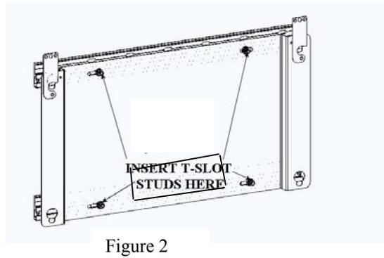
1. Install the four threaded studs into the four T-slot nuts.
