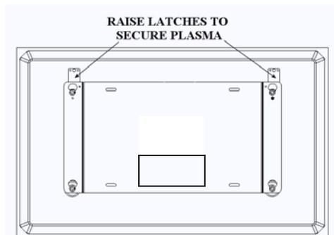
1. Place mounting buttons on mounting holes and attach using M8-1.25 x 35 mm BHCS (Figures 2 & 3).
