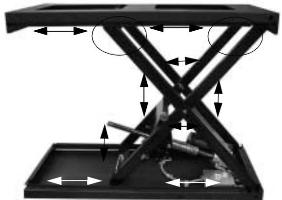
Figure 2. Examples of Pinch Points
