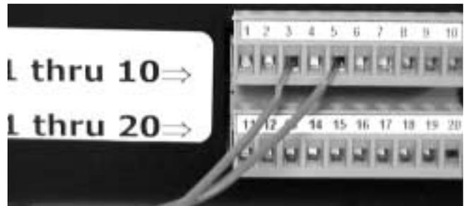
Figure 14. 12 Volt internal Supply Jumper
