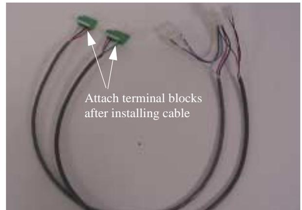
Figure 8. Optional Circuit Board Cable (with Terminal Blocks attached)
