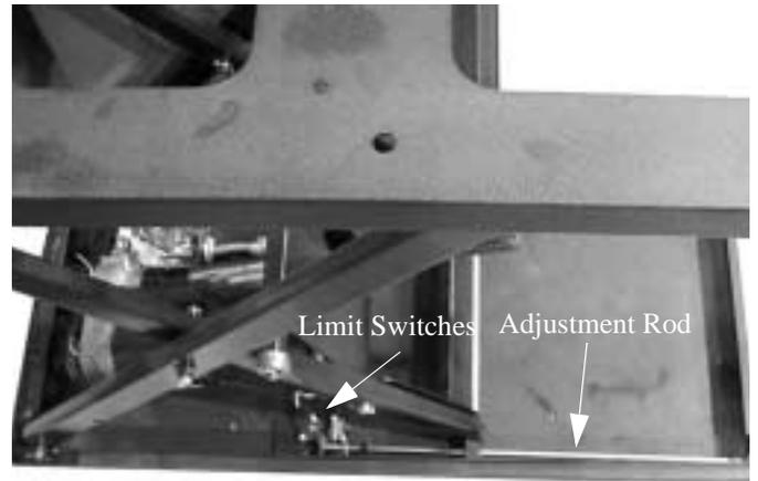
Figure 5. Adjustment Rod Location
