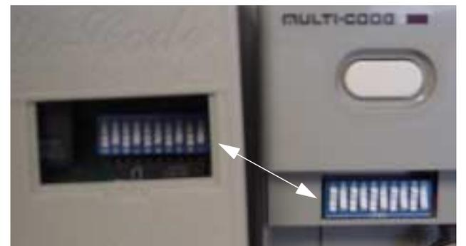
Figure 21. Dip Switches
