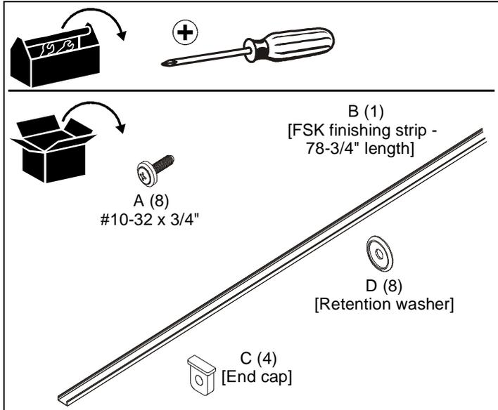
5. Install retention washers (D) onto #10-32 x 3/4" Phillips screws (A). (See Figure 2)
