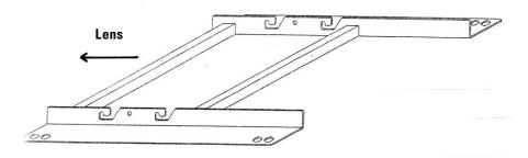
The overhead support **must** be capable of supporting **five times** the weight of the mount **and** equipment combined. If it cannot support this weight, the ceiling **must** be reinforced.
