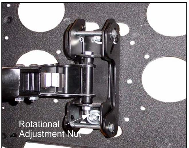
Figure 14: Rotational Adjustment
