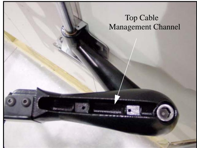
**Figure 8: Cable Management Channel (Top)**
