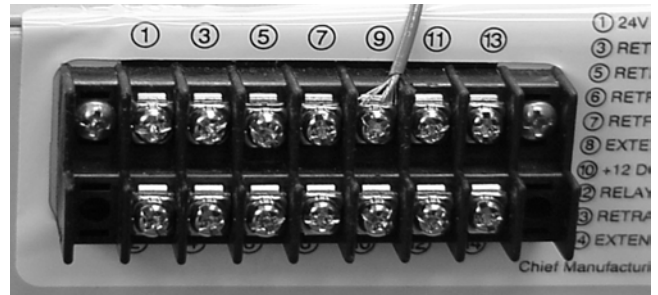
Figure 2. Green Wire to Terminal #9
