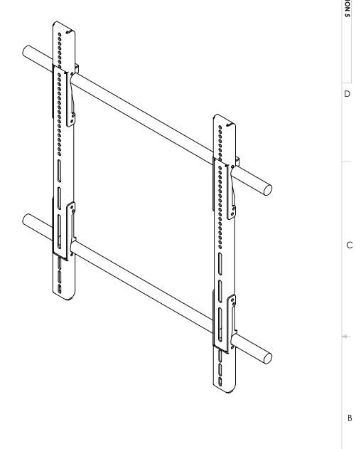
OPTION TO USE BRACKET EXTENSIONS WHEN HEIGHT IS 18.50" - 27.50" (469.9 mm -698.5 mm)
