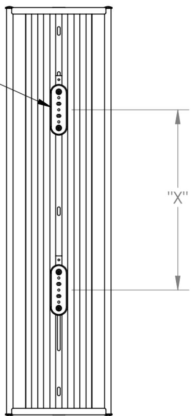
MINIMUM DISTANCE BETWEEN COMPONENT MOUNTING BRACKETS IN VERTICAL CONFIGURATION
