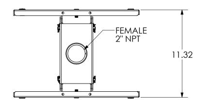
NOTE: CUSTOM INTERAFCE BRACKET NOT SHOWN. THE CUSTOM INTERFACE BRACKET NEEDED FOR YOUR DISPLAY WILL ADD BETWEEN 1/2" AND 2" IN DEPTH AND MAY AFFECT LOCATION OF DISPLAY ON THE MOUNT.
